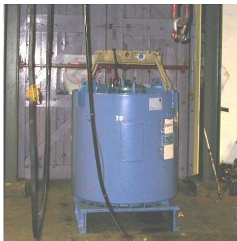
FIG. 1. Type B(U) packaging container for cobalt-60 sources.
